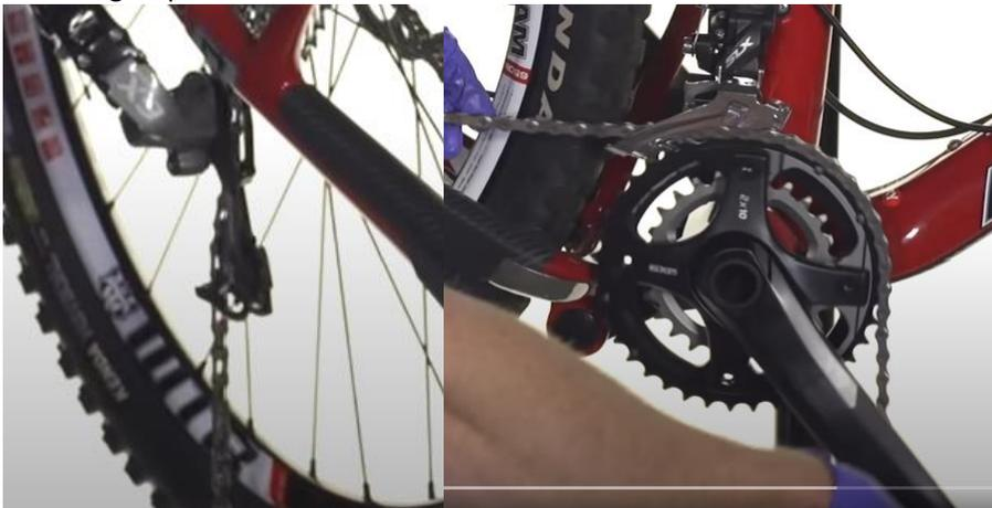
4. Insert the pins of each side of the master link into the ends of the chain.
