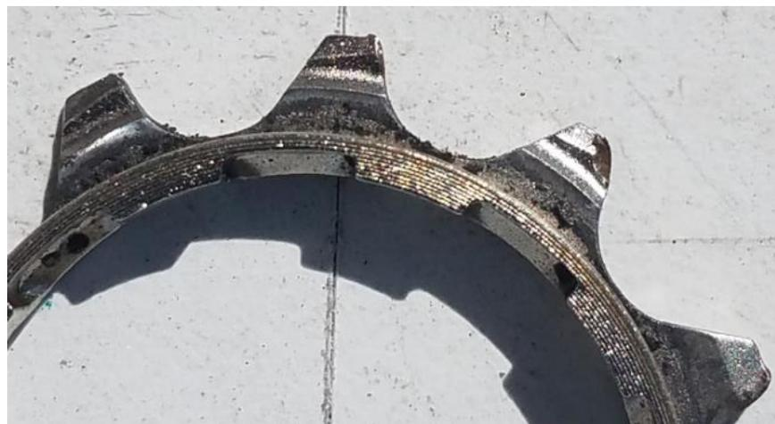
*Same cog after three miles of acceleration from a full stop in 10<sup>th</sup> gear using power level 5. Note tooth damage. Also prior Shimano version of Cassette.*
