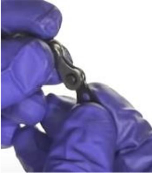
5. Pull the chain together and align the pins with the slots on the master link plates.
