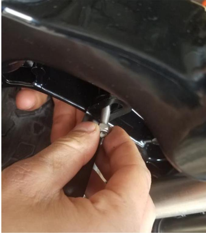
5. Use an adjustable wrench or 10 mm socket wrench to secure the nut.
