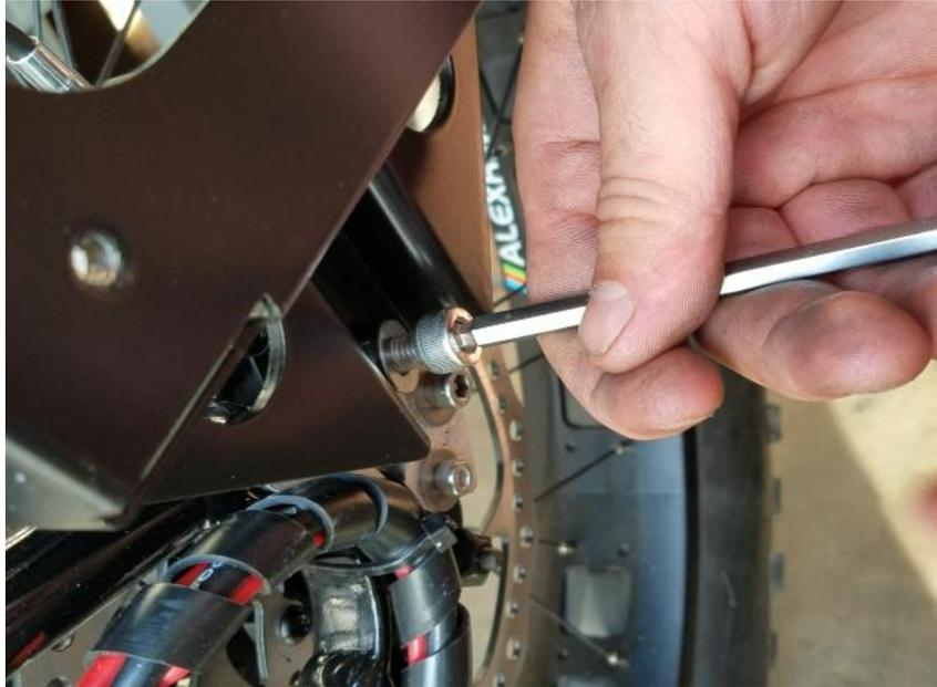
6. Align the holes in the tab at the bottom right side of the rack with the fastening location on the right-side metal rack support. Thread an M8 screw and washer through the tab and into the rack support. Finger tighten the screw.
