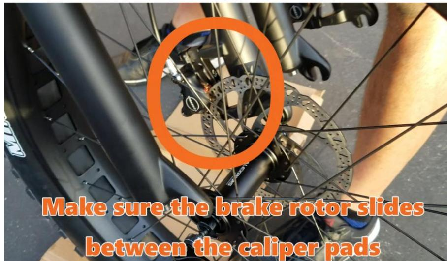
25. The ends of the axle will sit in the fork “dropouts” when correctly aligned. You may have to unscrew the end cap a turn or two if the fork doesn’t drop in place.
