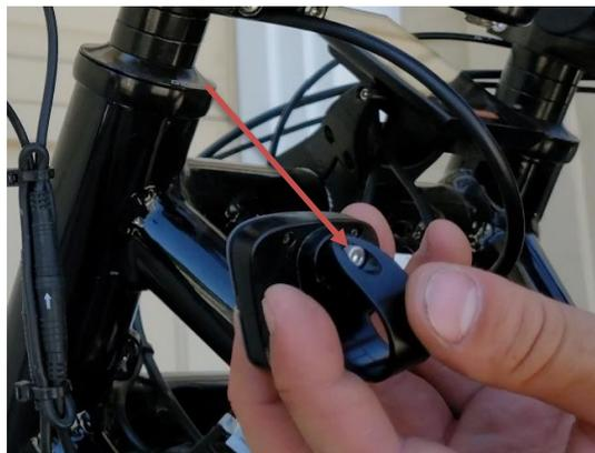
14. Mount the keypad onto the left handlebar and slide the keypad near the throttle.
