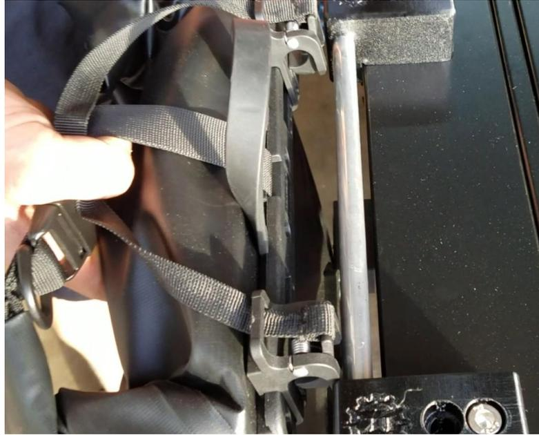
3. Push down on the pannier while pulling up on the quick release strap. This opens the two catches so that they engage the upper mounting tube.
