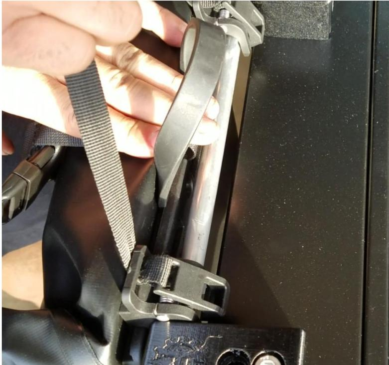
4. Lower the pannier onto the upper mounting tube and let go of the quick release strap. This locks the pannier in place.
