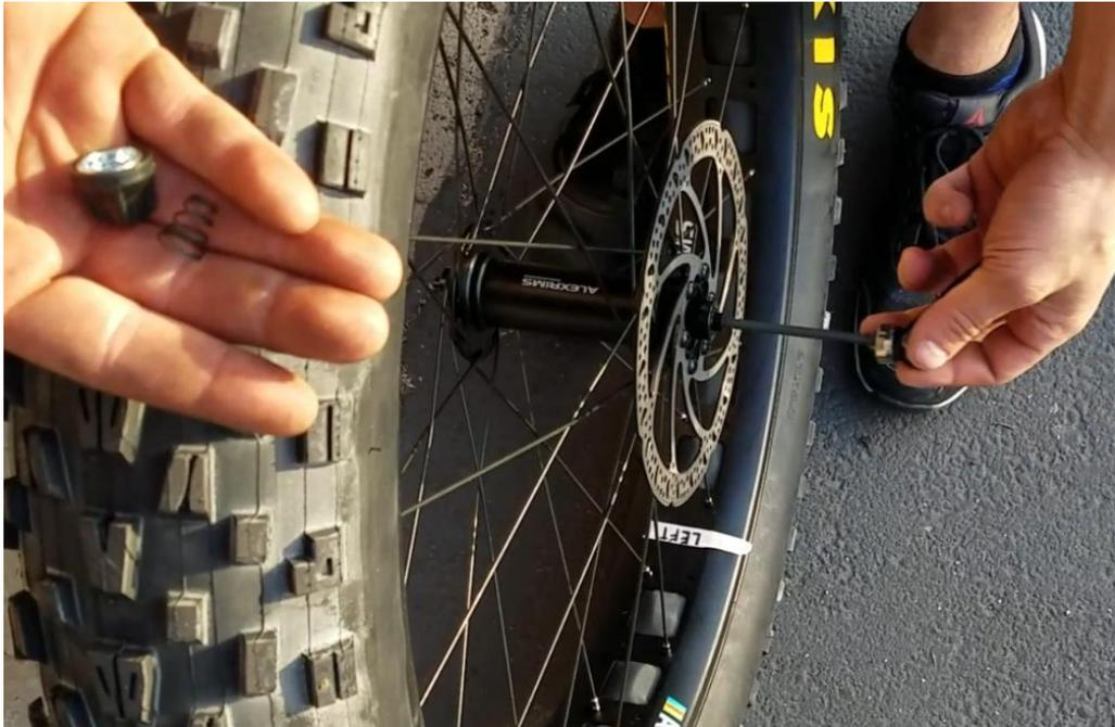
20. Replace the conical spring (small end first) on the other side of the wheel. Screw the end cap on a few turns to ready the wheel for installation.
