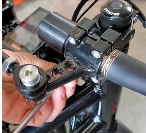
10. From the front of the bike, align the handlebar by rotating it so the middle hash-mark (7<sup>th</sup>) lines up with the upper inside edge of the stem as shown below.
