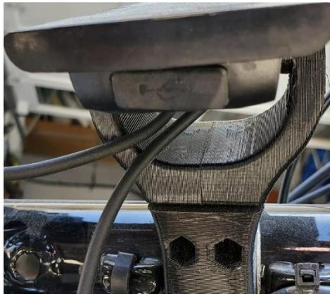
You can charge your phone or power a GPS unit with a standard USB charging cable.
