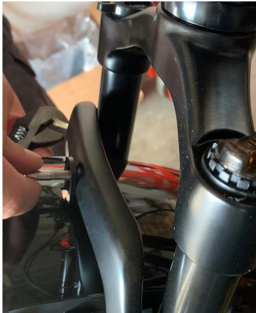
4. Thread the nut onto the back of the screw behind fork bridge.
