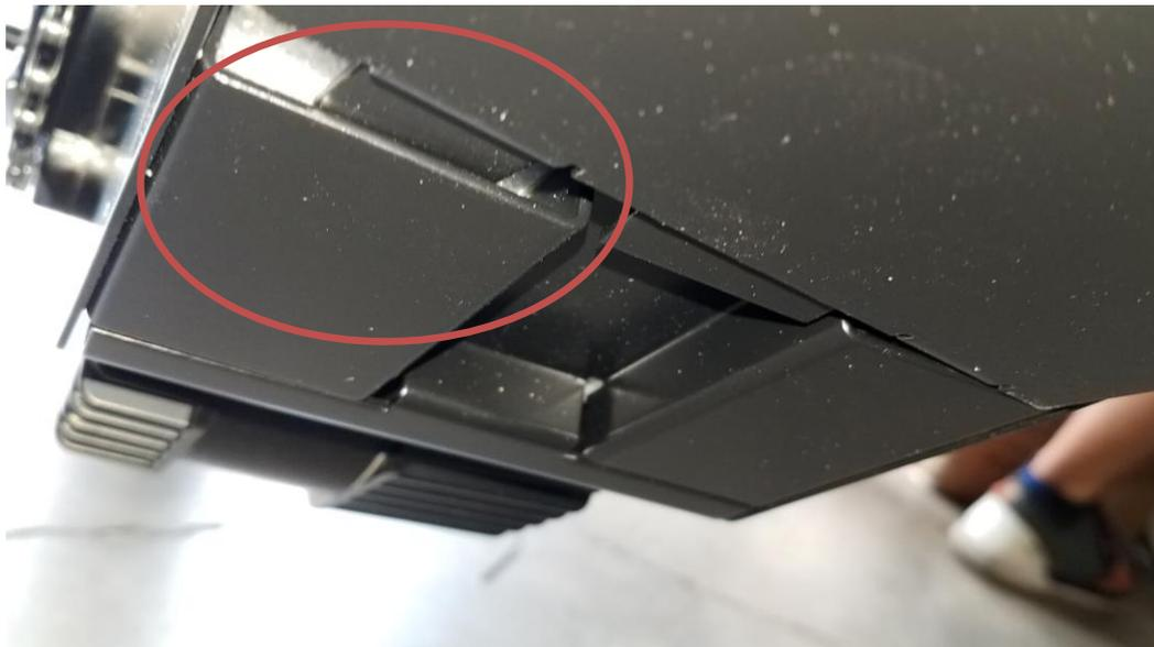
9. Push the cover closed making sure not to pinch any cables or battery padding.
