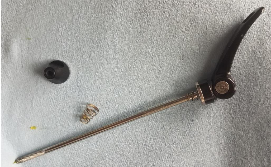
19. Insert the skewer into the LEFT wheel from the side of the brake disc as shown below.
