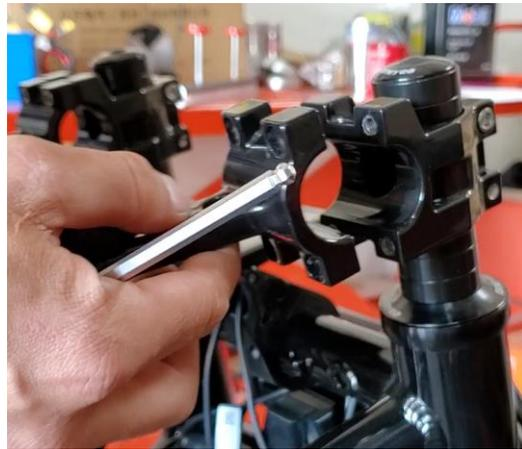
8. Place the right-side handlebar in the clamp such that there's a 1/8" gap between the handlebar end stop and the side of the stem as seen from the front of the handlebar.
