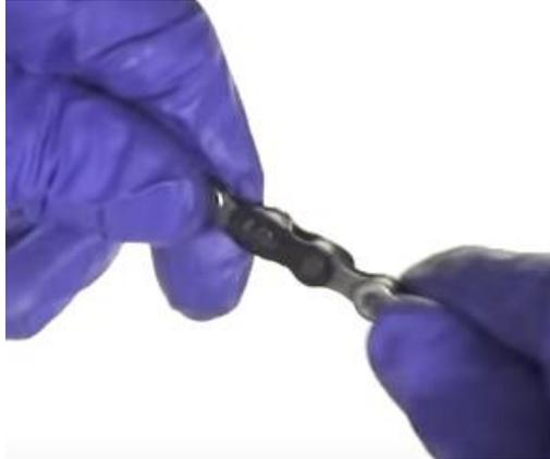
6. Rotate the chain so that the master link is above the chainstay and on the chain ring. With the rear brake engaged, you can step or use your hand on the right-side pedal to pull on the chain and set the master link. You should feel the master links “click” into place. Rotate the chain to verify the master links are set.
