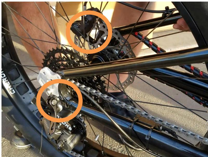
3. Make sure the wheel axle is seated in the left and right dropouts, then carefully lower the wheel onto the ground. Gravity helps seat the axle in the dropouts. Then, tighten the quick release end cap. As a guideline the end cap nut should begin to clamp onto the left drop out when the quick release lever points away from the wheel at a right angle.
