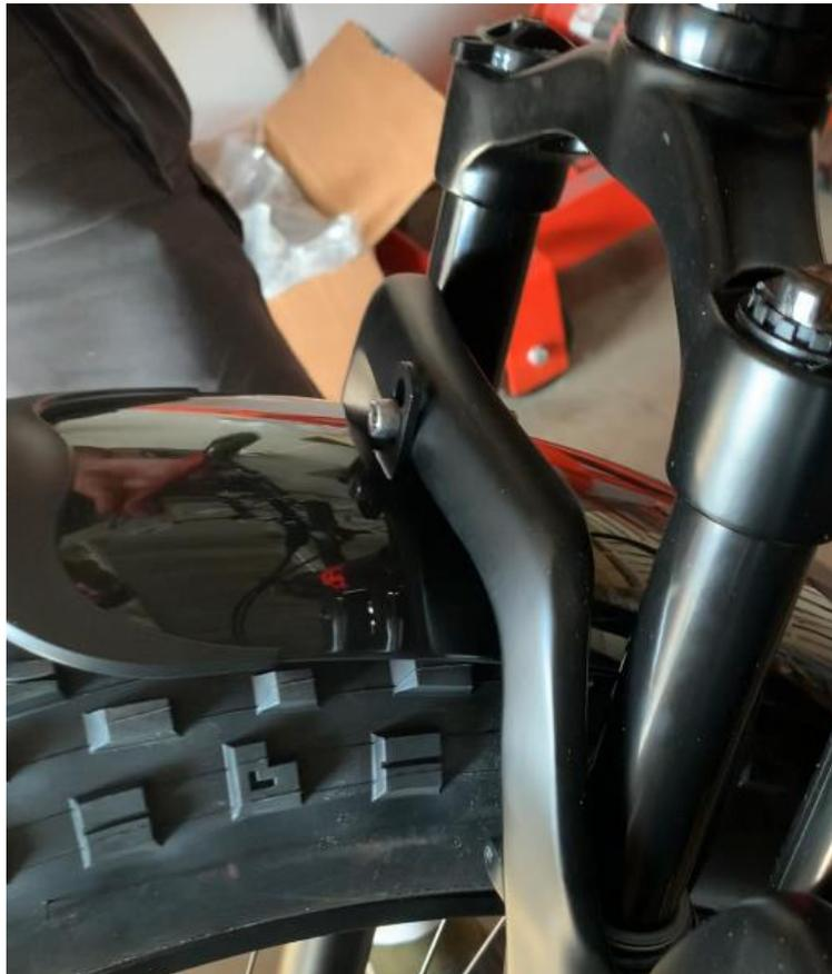
8. Adjust the mud flap to align it with the tire and fully tighten the nut.
