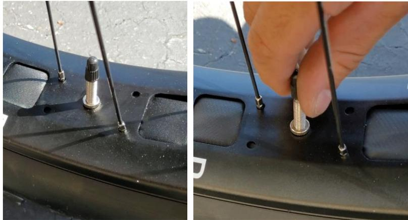
2. Unscrew the captive nut on the top of the presta valve to allow air to flow into the tire.
