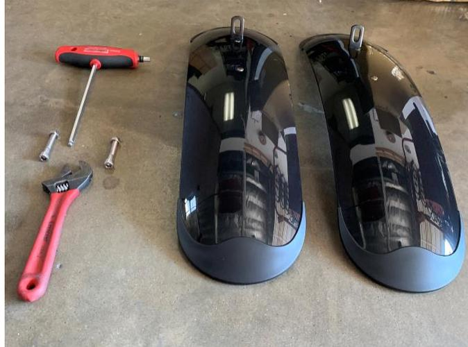
1. Remove the mud flaps from packaging along with their screws and retention nuts. Remove the retention nut from each screw. You'll need a crescent wrench (or 10 mm socket wrench) and a 5mm hex wrench to install the fenders
