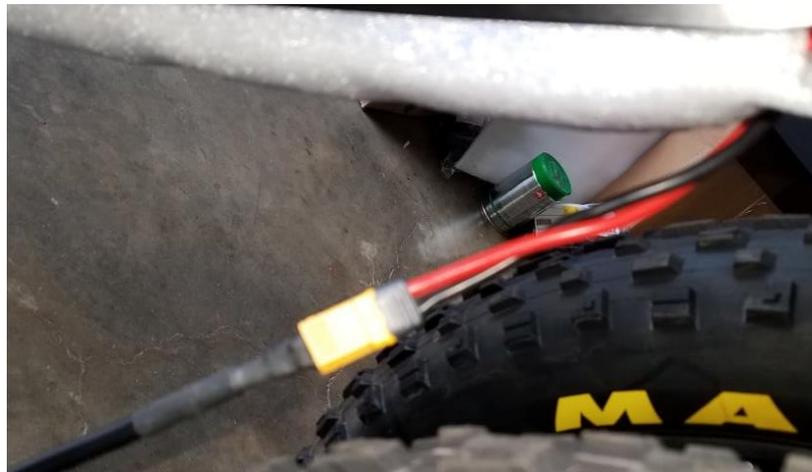
**NOTE:** You may hear a “pop” sound when you plug in the charger that comes from a spark that occurs inside the connectors when the two connectors mate. This is normal and a result of the potential difference between the battery and the charger.
