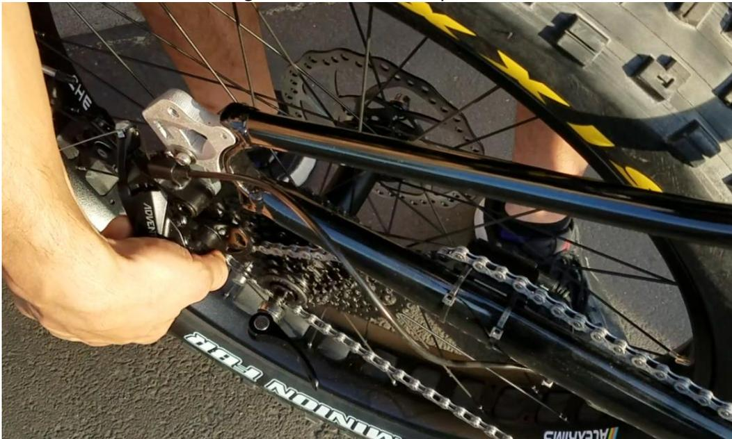
7. Move the chain above the cassette so it doesn't interfere with wheel removal.
