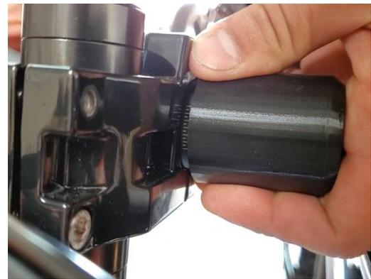
9. Replace the four bolts in the handlebar clamp and finger tighten.
