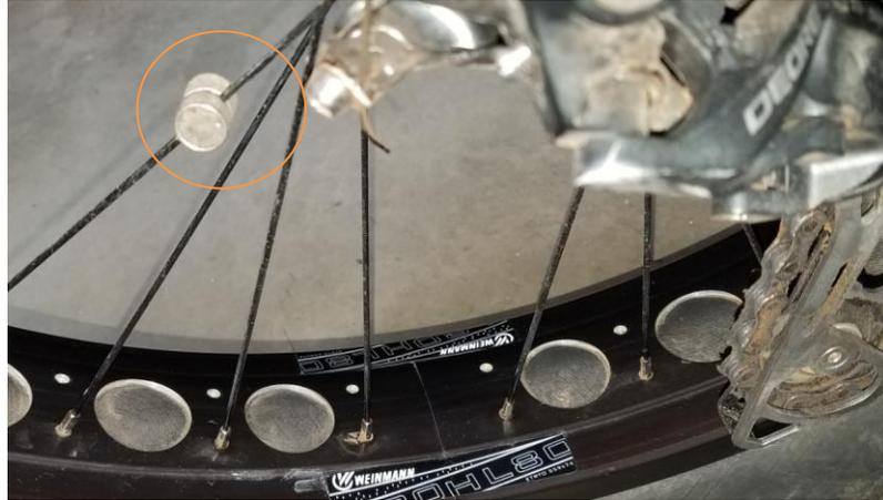
4. If you are replacing a magnet, place the magnet so that the face of the magnet faces the sensor and aligns with the oblong recess on the sensor – it has the word “Bafang” embossed.
