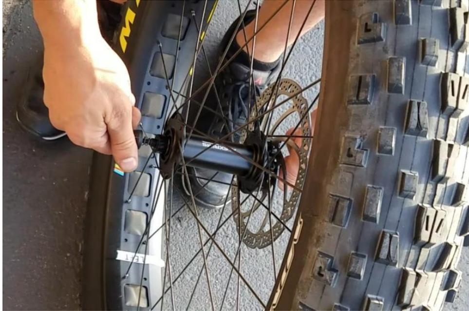
21. Prep the RIGHT wheel. Insert the other skewer into the RIGHT wheel from the side OPPOSITE to the brake disc as shown below.
