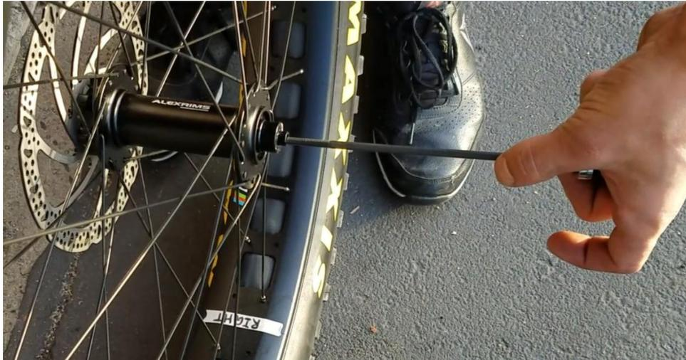
22. Replace the conical spring (small end first) on the other side of the wheel. Screw on the end cap with a few turns to ready the wheel for installation.
