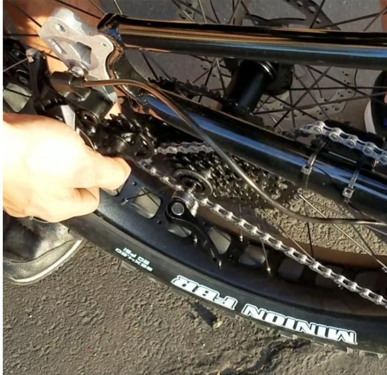
2. Remove any support for the frame and lower the frame so the axle of the wheel moves up into the dropouts. Take care to slide the brake rotor between the brake caliper pads on the left side of the bike.
