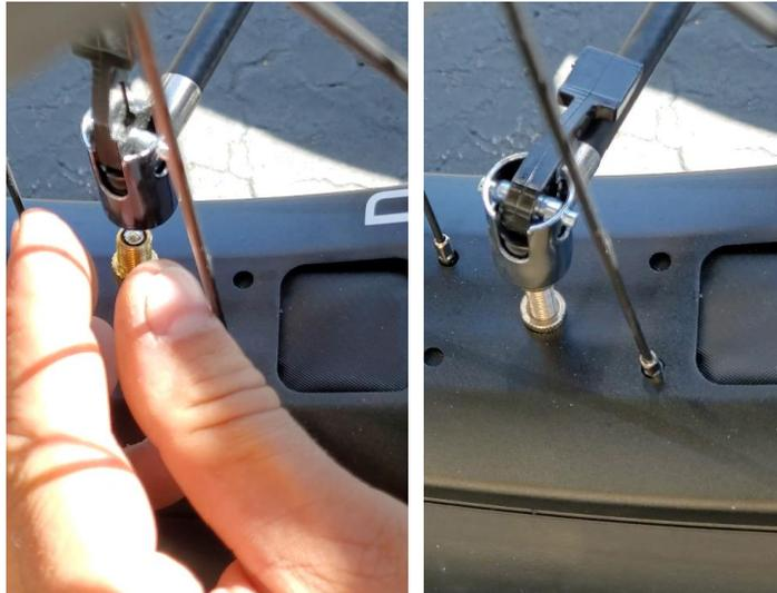
5. Remove the bike tire pump and unscrew the Presta valve adapter. Put the valve adapter in a safe place; they are easy to lose.
