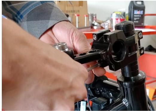
7. Open the right-side handlebar clamp to allow placement of the right-side handlebar.
