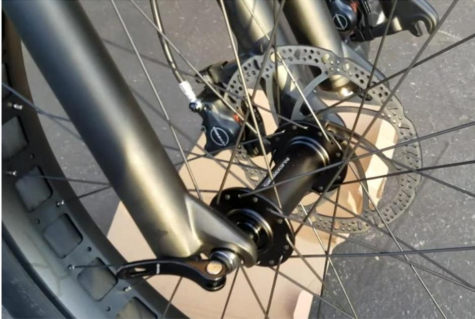
26. Tilt the bike and mount the LEFT wheel to the LEFT fork making sure that the rotor fits between the brake caliper pads.
