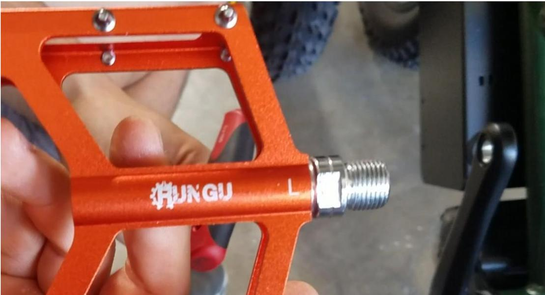
34. Use your fingers to thread the pedal shaft by inserting the threaded shaft into the crank arm. Then hold the threaded section of the pedal in the crank arm mounting hole and spin the entire crank arm in a clockwise motion as depicted below.
