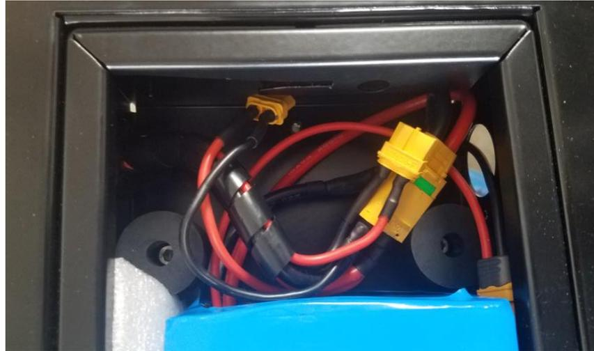
*GOOD - cables placed away from door and key latch*
