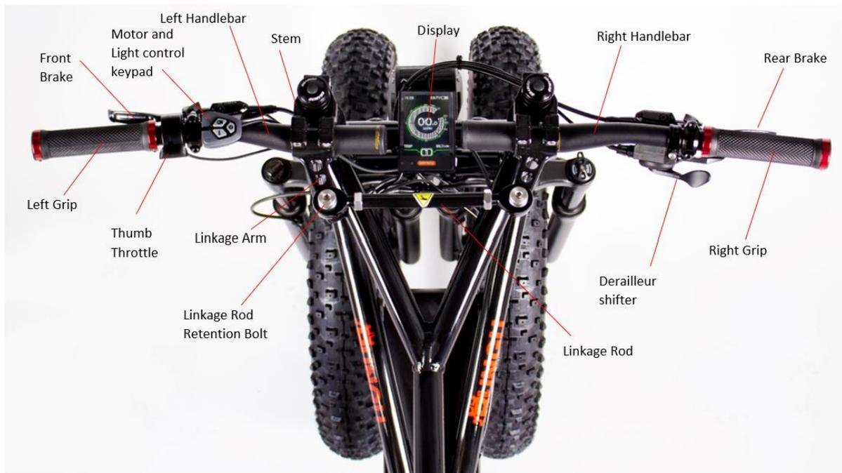
Figure 2 Steering assembly
