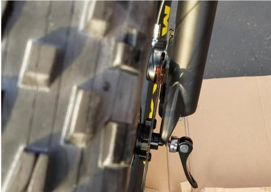
27. The ends of the axle will sit in the fork “dropouts” when correctly aligned. You may have to unscrew the end cap a turn or two if the fork doesn’t drop in place.
