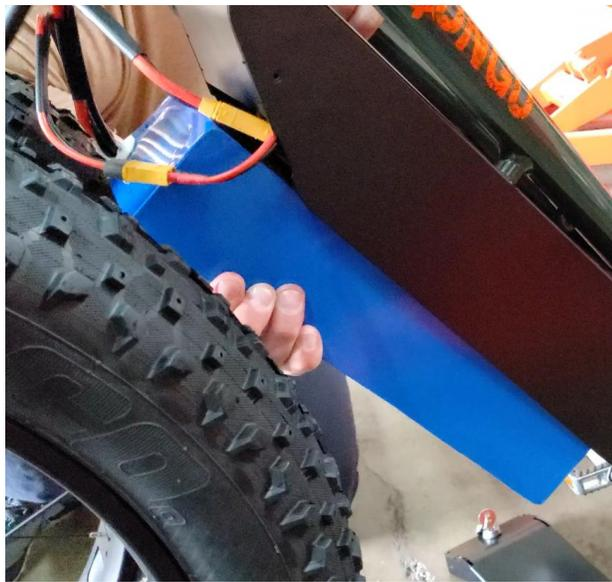
**CAUTION: IF YOU DECIDE TO REMOVE THE BATTERY, MAKE SURE YOU HAVE THE GRIP AND ARM STRENGTH TO REMOVE IT – THE BATTERY WEIGHS APPROXIMATELY 10 LBS. (4.5 KGS).**
