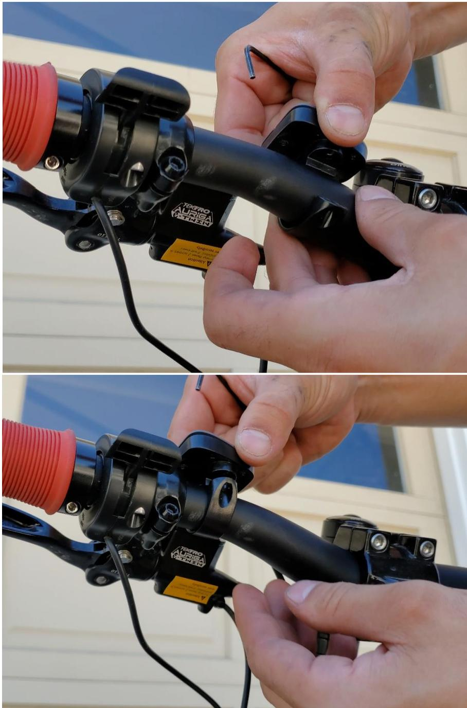
15. Reinsert the retention screw and tighten so the keypad doesn't rotate on the handlebar.
