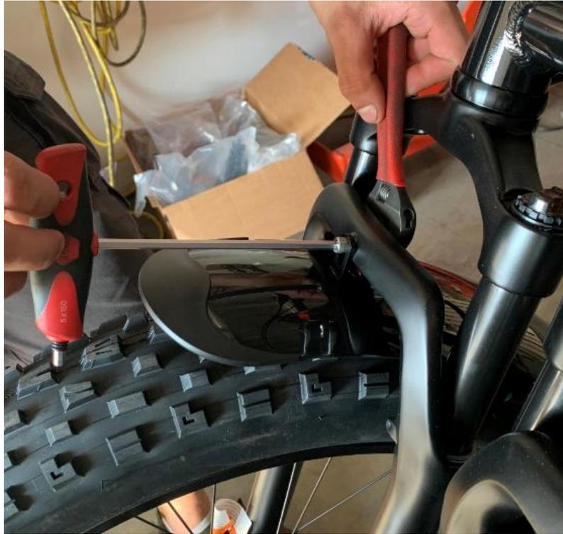
7. Before fully tightening the nut, slide the mud guard up vertically to maximize wheel clearance.
