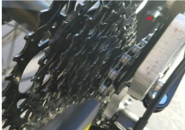
2. If possible, find an object (e.g. empty bucket, cardboard box) that you can use to support the bike after the rear wheel is removed. Alternatively, hang the rear triangle from straps or ropes to support the rear triangle after the rear wheel is removed.
