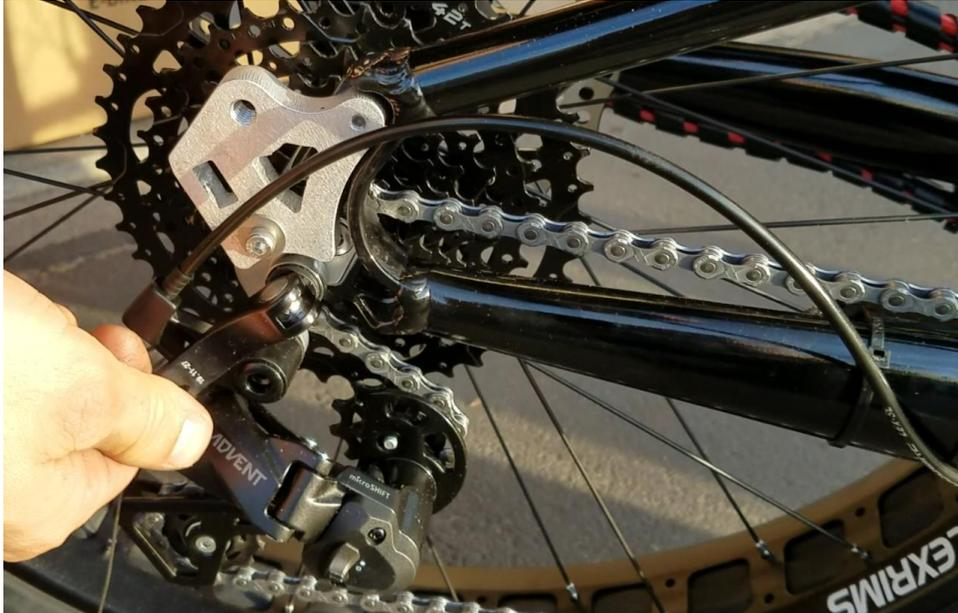
4. Loosen the quick release skewer by unscrewing the end cap. Be careful to not lose the springs or other components of the skewer if you remove the end cap.
