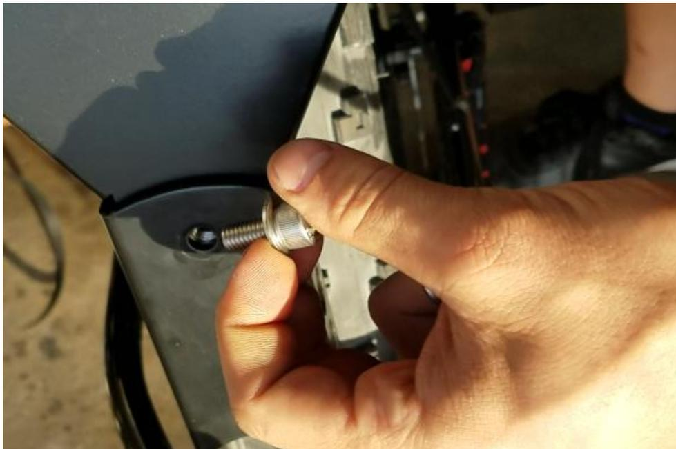
5. Align the holes in the tab at the bottom left side of the rack with the fastening location on the left side metal rack support. Thread an M8 screw and washer through the tab and into the rack support. Finger tighten the screw.
