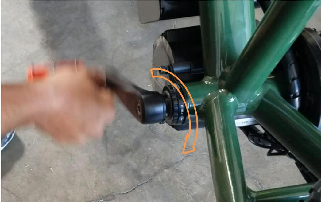
35. Use a 6mm Hex wrench to tighten the pedal once the pedal is fully inserted.
