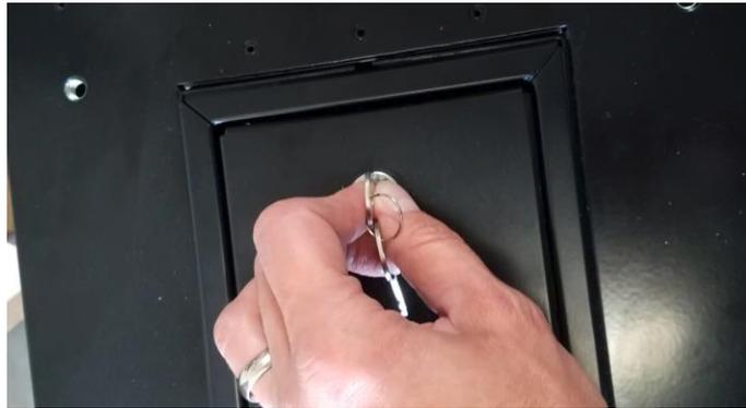
**Caution:** The battery has padding inside of the rack to minimize shock and vibration; turning the key may require that you overcome the pressure from this padding. Do not remove the padding from the battery.
