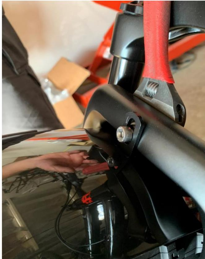
6. Use a 5mm hex wrench to continue threading the nut onto the screw
