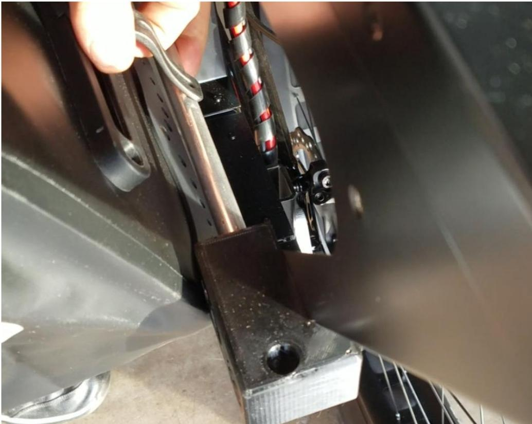
2. Adjust the upper quick-release catches using the adjustment knobs so that the catches fit between the two upper mounting blocks.
