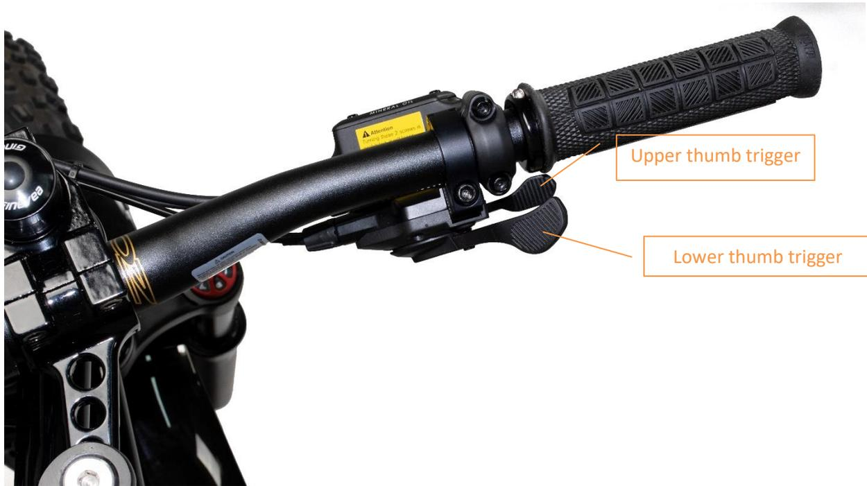
Each press of the thumb against one of the triggers indexes the gear. A long press of the Lower Thumb Trigger decreases the gear by one gear at a time starting in ninth gear. A short press of the Upper Thumb Trigger increases the gear by one gear at a time starting with first gear.
