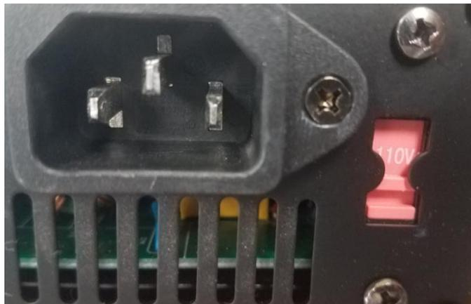
If the voltage input switch is set incorrectly for your voltage standard, use the blade of a small screwdriver to push the switch to the correct setting.
